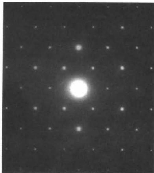
Fig. 1. An hhl electron diffraction pattern from C 60 buckminsterfullerene [111] plates tilted 35^\circ around the \mathbf{d}_{110}^* reciprocal axis. Note that these patterns, which are obtained from crystals grown by evaporation of a dilute solution of the material in benzene, do not have the twinning characteristics described by Ishiguro & Hirotsu (1992).
